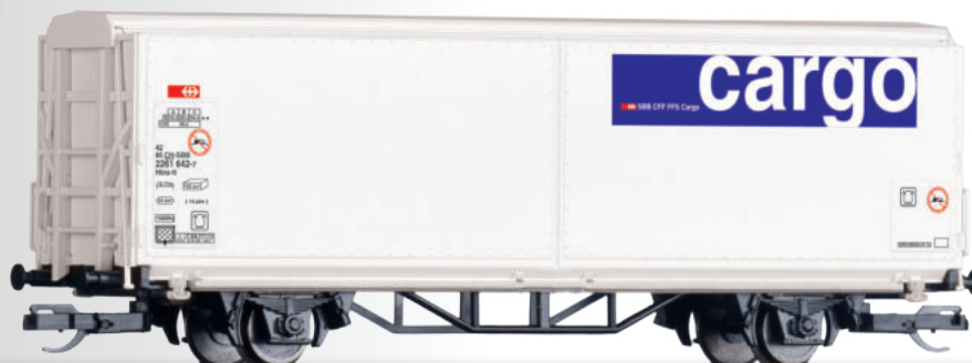
Schiebewandwagen Hbis-tt der SBB Cargo Sliding wall box car Hbis-tt of the SBB Cargo
